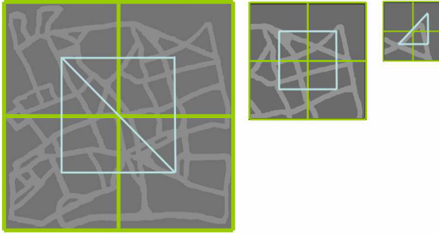
Fig. 2. Illustration of different levels of hierarchy of a quad-tree applied on an environment as shown in dark green. On the left hand side is shown the highest level, while the subsequent subdivision of the NE corner is shown on the right hand side. In light blue is shown the new graph structure built from the quad-tree, with cells linked only if there is at least one way to access directly one to another.
