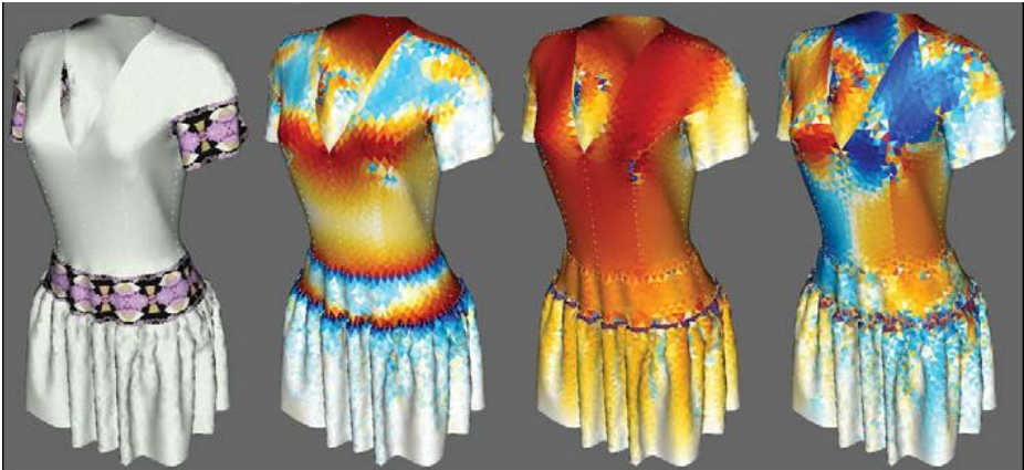
Fig. 5. Extraction of the weft, warp and shear tensile deformation values on the cloth surface using the 2D fabric surface coordinates of the patterns and the initial 3D shape of garment
